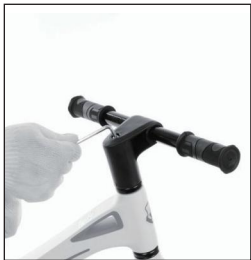
tighten the screw
