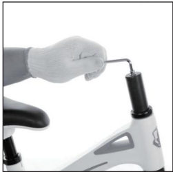
loosen the front fork tube screw
