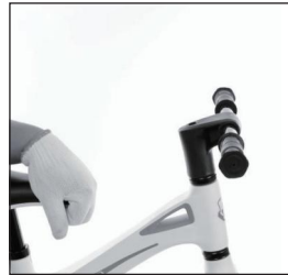
insert the handlebar to the front fork
