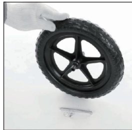
loosen the wheel screw
