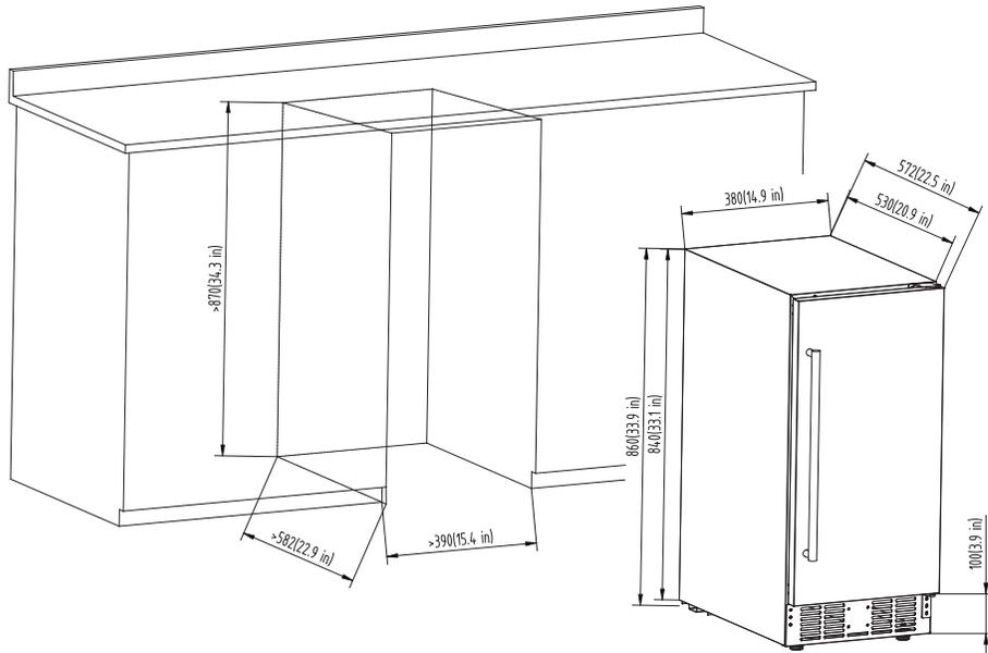
For freestanding installation, suggest to allow 2 inches of space between the unit's side, rear and the wall. In addition, sufficient clearance (160°) should be maintained to allow the door to open properly and completely.
