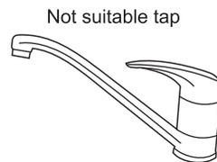
The front end should be longer than 0.4in. The tap exit end face should be flat and smooth, if not file it to avoid leakage.
