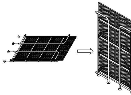
**EN:** Install the leveler at the bottom of the rack, and then put the rack upright.
