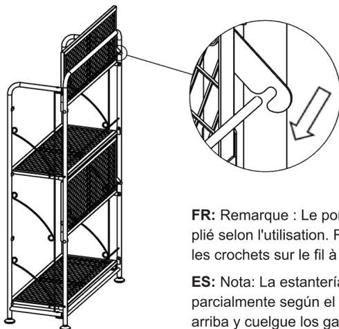
**EN:** Remark: The plant rack can be partially folded according to the usage. Fold the shelves up and hang the hooks on the wire at the back.
