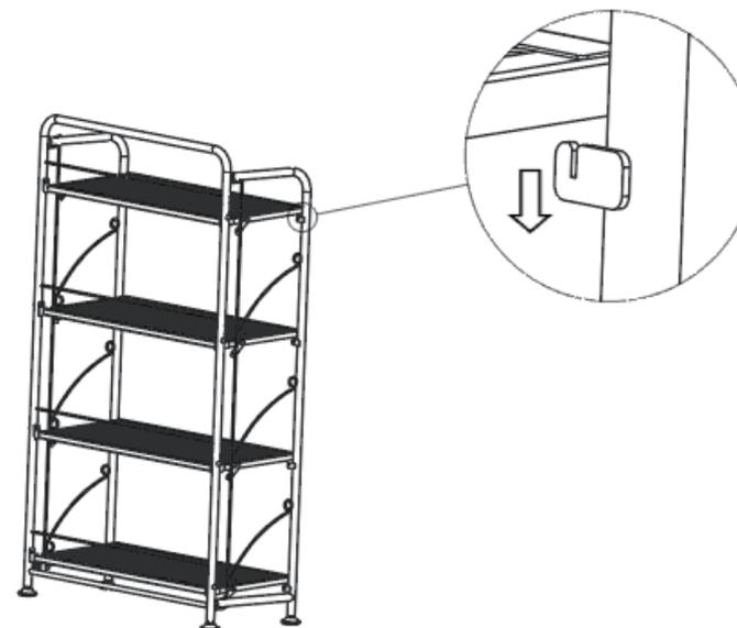
**EN:** Insert the bottom metal sheet on the shelves into the buckle of the both side frames, pay attention to fixing both sides at the same time.
