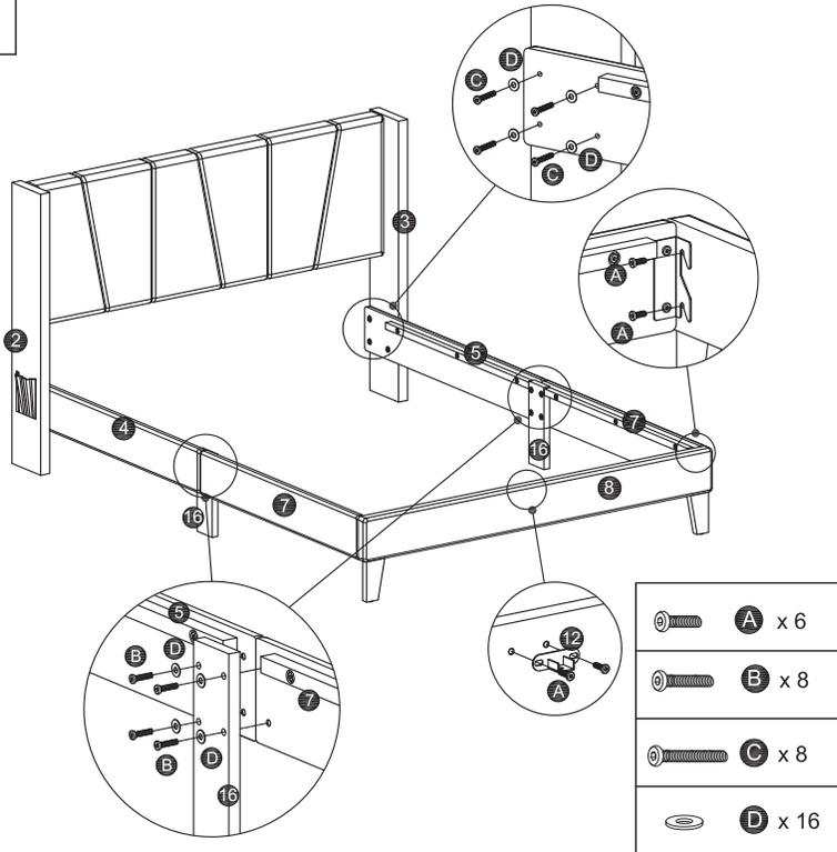
**EN:** Attach Part (4,5) to Part (2,3) with Bolt (C) and Washer(D) using Hex Key(E).
