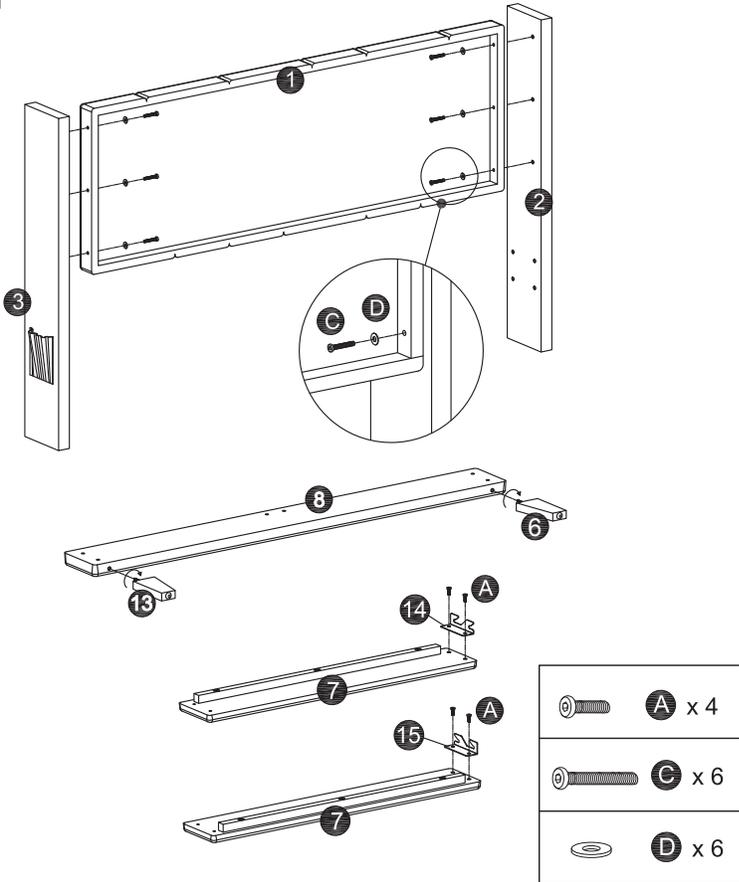
**EN:** Attach Part(2,3) to Part(1) with Bolt(C) and Washer(D) using Hex Key(E).
