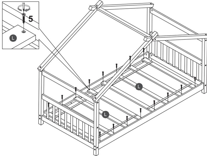
**EN: Note:** Do not lock the screws of the bed slats to the outermost edge of the bed slats, you need to leave a certain space at the edges, otherwise it will cause the board to break.
