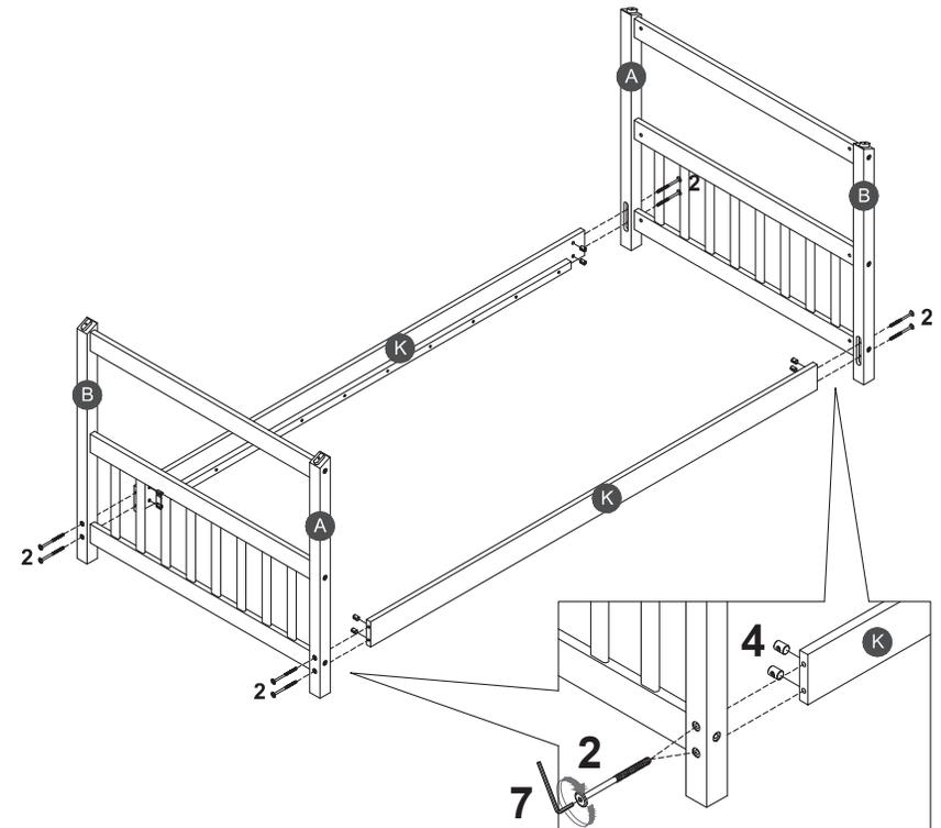
**EN:** Note: Part 4 will face up with the "x" mark on it, otherwise it cannot be tightened.
