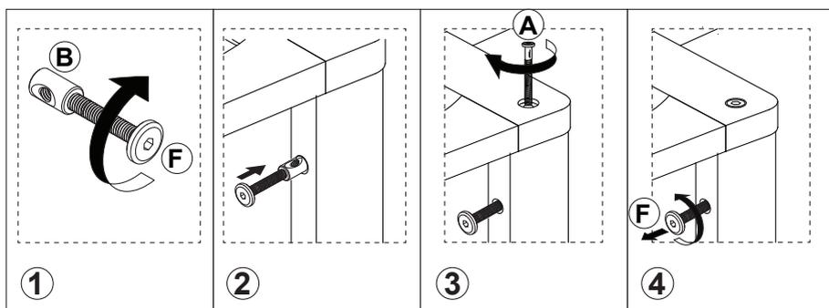
**EN:** ① Fix and tighten Bolt (F) into Cross dowel (B).
