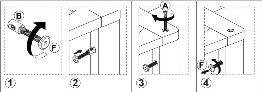
**EN:** ① Fix and tighten Bolt (F) into Cross dowel (B).
