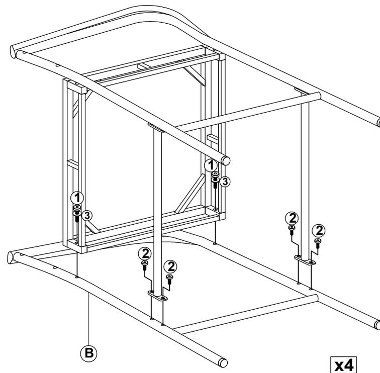
**EN:** Connect Assembly Part from STEP 1 to Left Leg Frame (B) with Bolts (1), (2) & Washers (3).
