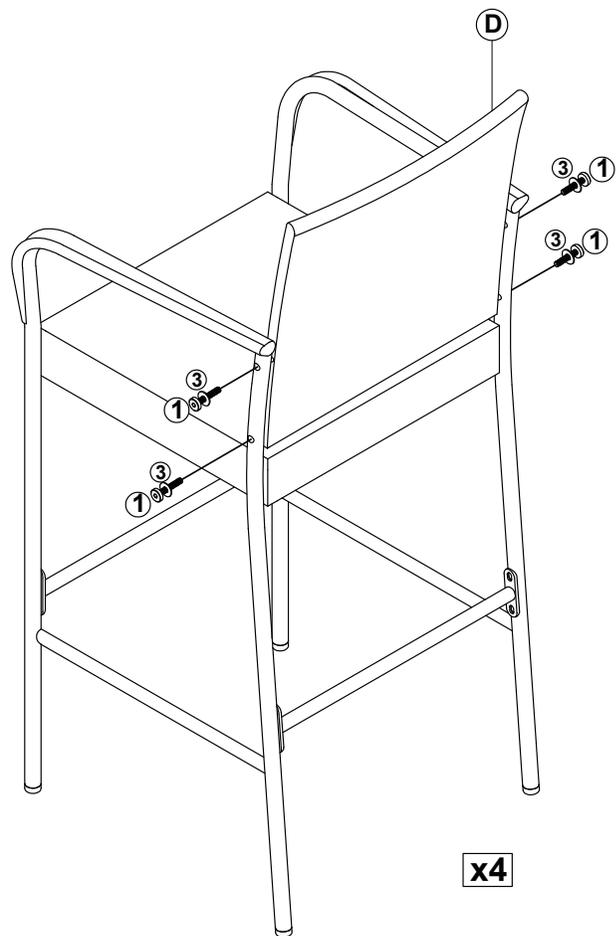
**EN:** Connect Assembly Part from STEP 2 to Back Frame (D) with Bolts (1) & Washers (3).
