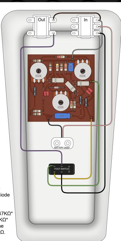
All three transistors are germanium PNP. The diode is germanium.
