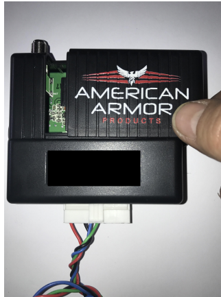
Remove cover by sliding dip switch access door to the right
