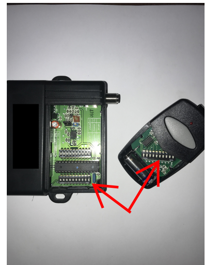
Set dip switch code on receiver to match transmitter and replace covers
