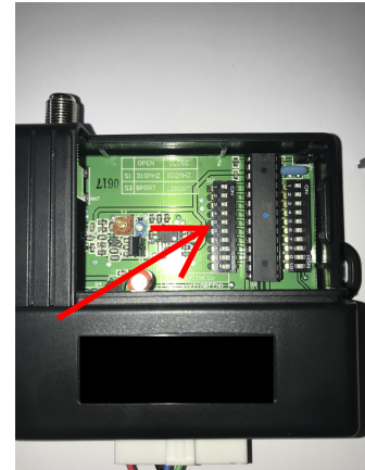
Set dip switch code on left to match transmitter
