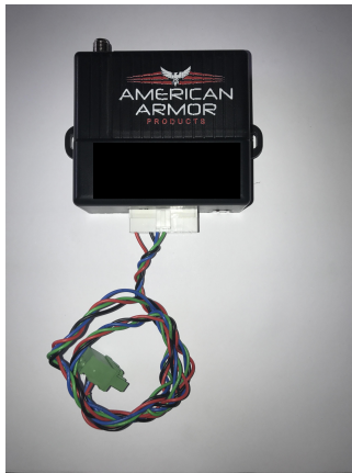
Ranch Code Receiver pre-wired with circuit board plug
