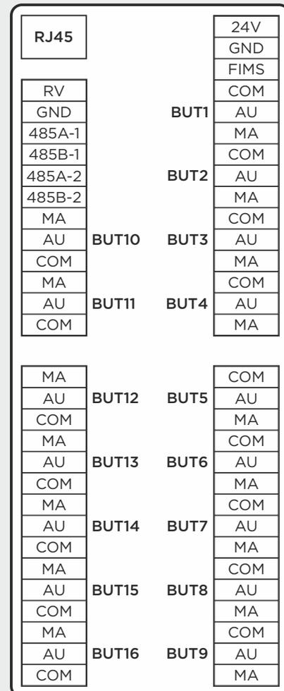
To connect the relay contacts of each floor you need to use the contacts **MA** and **COM**.
