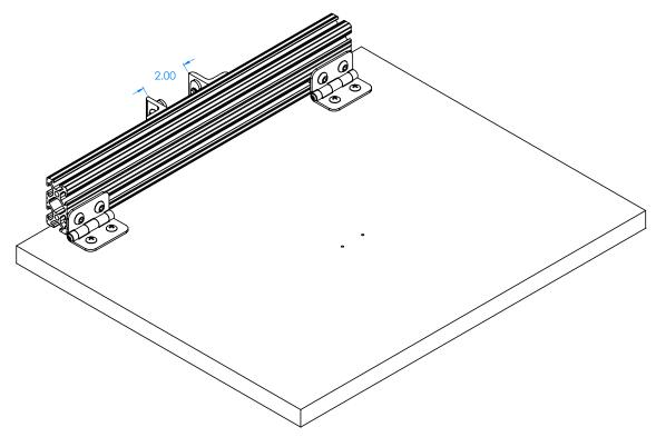
ASSEMBLE ALL COMPONENTS ON A FLAT SURFACE TO ENSURE ALL JOINTS ARE SQUARE AND NOT TWISTED. IF JOINTS BECOME TWISTED WHEN TIGHTENING SCREWS, IT WILL THROW OFF THE CALIBRATION IN LATER STEPS.
