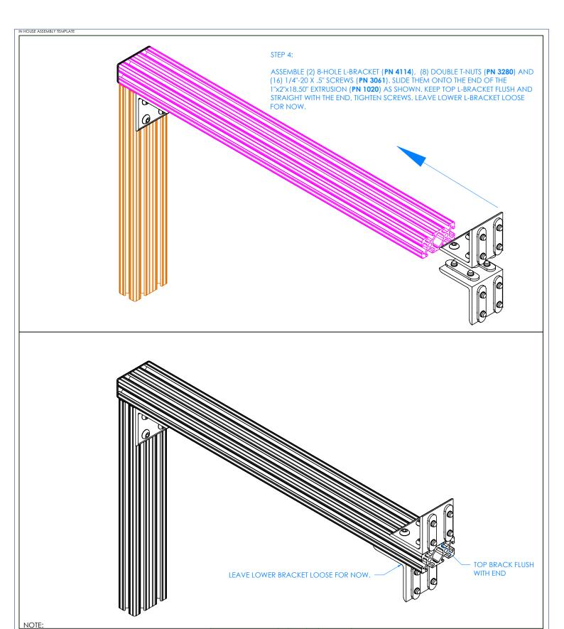
ASSEMBLE ALL COMPONENTS ON A FLAT SURFACE TO ENSURE ALL JOINTS ARE SQUARE AND NOT TWISTED. IF JOINTS BECOME TWISTED WHEN TIGHTENING SCREWS, IT WILL THROW OFF THE CALIBRATION IN LATER STEPS.
