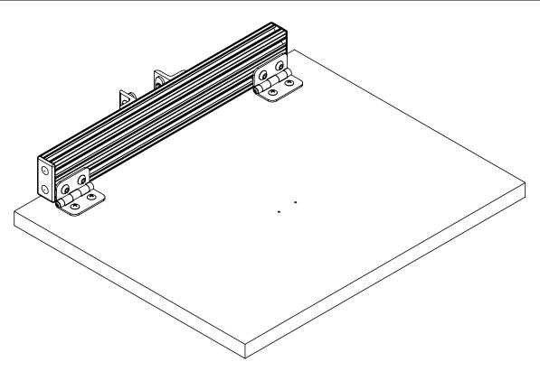
ASSEMBLE ALL COMPONENTS ON A FLAT SURFACE TO ENSURE ALL JOINTS ARE SQUARE AND NOT TWISTED. IF JOINTS BECOME TWISTED WHEN TIGHTENING SCREWS, IT WILL THROW OFF THE CALIBRATION IN LATER STEPS.
