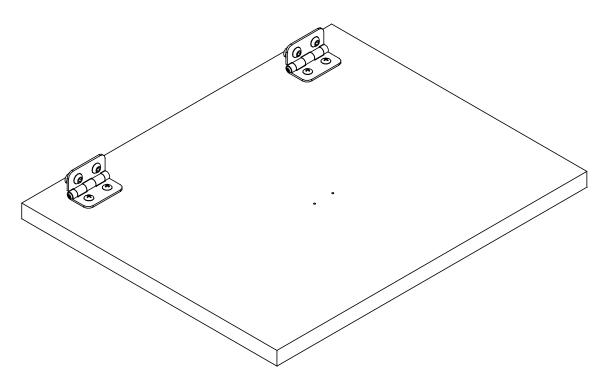
ASSEMBLE ALL COMPONENTS ON A FLAT SURFACE TO ENSURE ALL JOINTS ARE SQUARE AND NOT TWISTED. IF JOINTS BECOME TWISTED WHEN TIGHTENING SCREWS, IT WILL THROW OFF THE CALIBRATION IN LATER STEPS.
