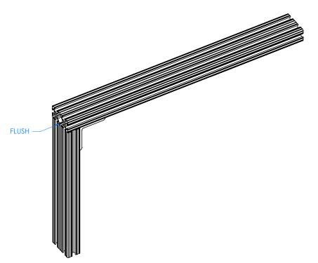
ASSEMBLE ALL COMPONENTS ON A FLAT SURFACE TO ENSURE ALL JOINTS ARE SQUARE AND NOT TWISTED. IF JOINTS BECOME TWISTED WHEN TIGHTENING SCREWS, IT WILL THROW OFF THE CALIBRATION IN LATER STEPS.
