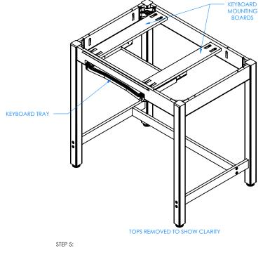
IF YOUR TABLE DOES NOT HAVE A KEYBOARD TRAY OR CPU SUPPORT SKIP TO STEP 8. ATTACH KEYBOARD TRAY TO THE TWO KEYBOARD MOUNTING BOARDS WITH THE HARDWARE PROVIDED. NOTE: IT MAY BE EASIER TO ATTACH KEYBOARD TRAY WHILE TABLE IS ON 11S TOP. ATTACH THE MONITOR POST TO THE TOP USING HARDWARE PROVIDED (NOT SHOWN).
