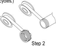
3. Screw pipe into bushing.
