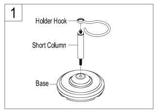
1. Place base on a solid level surface and thread in short column in a clockwise direction. Insert holder hook onto top portion of short column.
