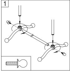
1. Screw in 29" vertical side bars into foot and bolt in bottom bar between assembly.
