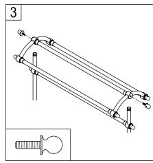
3. Bolt in top rack assembly to bottom assembly.
