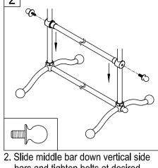
bars and tighten bolts at desired level.
