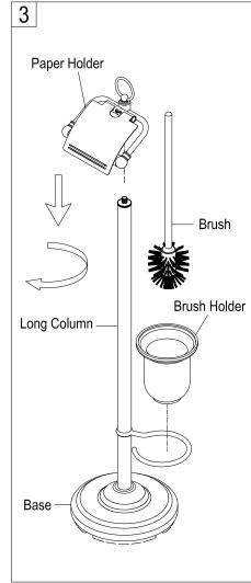
3. Thread paper holder on top of long column and insert spring loaded toilet paper holder bar. Insert Brush holder cup and brush.
