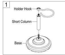
Place base on a solid level surface and thread in short column in a clockwise direction. Insert holder hook onto top portion of short column.
