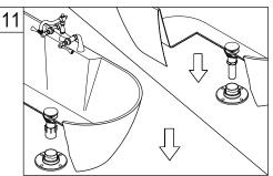
11. After Glue/ epoxy has been applied with the help of two or more people slowly pick up the tub and align the tub drain adapter to the drainage pipe, set tub in place.
