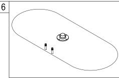
6. Rough in water supply lines on the side where the faucet will be situated, it is recommended that you install the shut-off valves for the faucets supply lines in a location easily accessible, and without having to remove the tub in case of leaks or faucet repairs.
