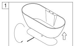
1. Position the tub at the desired location, with a pencil mark the perimeter of the tub, also mark the location of where the tub drain and faucet water supply lines will be situated, remove tub and place upside down on top of 2 pieces of lumber covered with a blanket or a piece of cardboard, the tub should be raised enough to allow for installation of the faucet.
