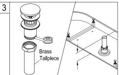
3. If you have access to the tub drain from below the floor, apply Teflon tape to the drain and thread the included tailpiece, measure the distance that it protrudes from the bottom of the tub and rough in your drain pipe accordingly.
