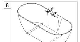
8. After placing 2 pieces of Lumber on the area where the tub will be installed, place the tub on top, add Teflon tape to the shut-off valves and attach the faucet supply lines.
