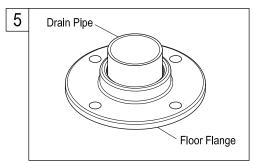
5. Secure floor flange to the area around the drain, this will serve as additional reinforcement to keep your tub drain in place in the event of any accidental impact on the tub.
