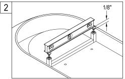
2. Adjust feet so that they protrude 1/8" below the level of the tub, you can accomplish this by placing a level or a straight piece of lumber across the width of the tub.
