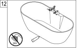
12. If you installed the tub using the drain tailpiece, with the drain still closed add more water into the tub, while inspecting the connections from below the floor, drain the tub and check for leaks, if you installed the tub using the drain adapter, allow the glue to dry for 24 hours before draining the tub, apply caulking around the perimeter as needed, clean off any excess caulking.
