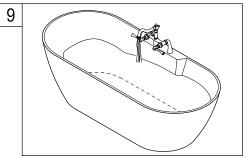
9. Close drain and open both hot and cold shut-off valves, open faucet valves and allow at least 1" to 2" of water into the tub, check for leaks on the faucet supply lines and drain.
