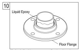
10. Apply liquid epoxy or a professional grade ABS glue or JB weld epoxy to the drain pipe coming from the floor, apply as per manufacturer's instructions.
