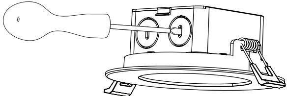
**5** Open the power supply box cover. Feed the supply wire into the knockout hole using a 3/8 in. clamp connector (not included) and make all the connections inside the power supply box using wago connectors. Connect the 120V line (black) wire to the black wire. Connect the neutral (white) wire to the white wire.
