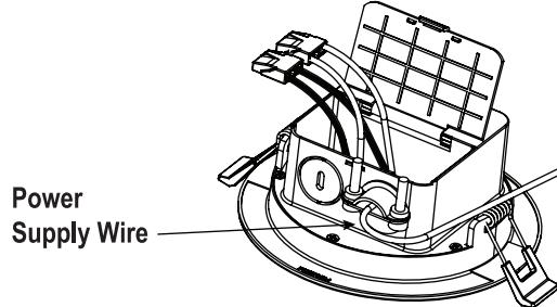
**6** After connecting the wires correctly, place the wires inside the power supply box and close the box properly.
