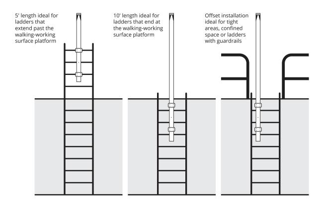
12" offset optimum solution for SRL attachment to back of harness D-ring, but can be used for sternal D-Ring attachment, too.
