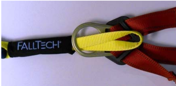
Fig. A-4 – Making Web-Loop Connections
