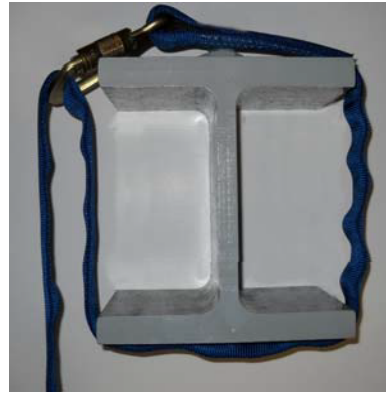
Incorrect Tie-Back Connection
