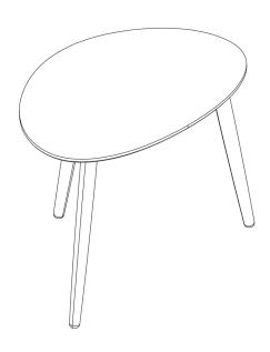
Lay the tabletop facedown on a flat, clean and non-abrasive surface. Attach the legs to the tabletop as shown in the diagram below. Tighten each leg by turn it clockwise.
