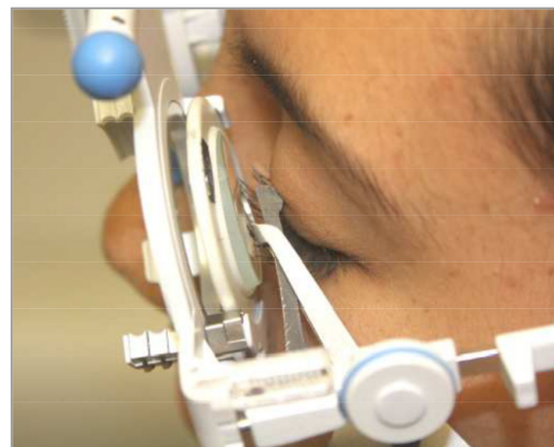
One end of the Distometer rests against the upper eyelid and the other contacts the rear of surface of the lens.
