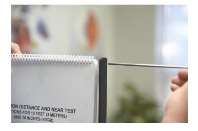
6. Line up the stainless steel rod to the hole on the top of the mounting bracket. Push through the top spiral bound of the Low Vision book and hole on the other side of the mounting bracket
