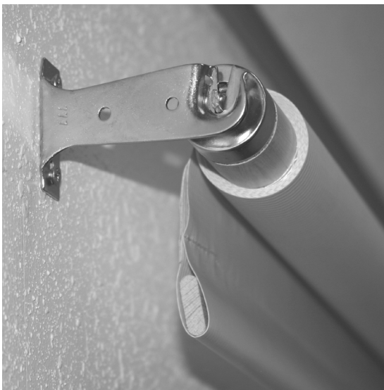
Left hand bracket, properly mounted showing slot for rectangular end of roller. Note how screen should roll off the back of the roller.
