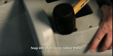
Step 4: Align the holes on the lower left riser with the mushroom caps on the lower step tread.
