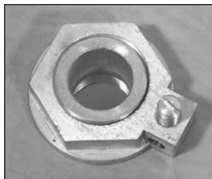
Threaded nut and bolt are not welded
