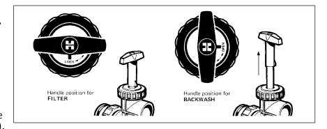
After backwashing, turn off pump. Push valve handle DOWN and turn to LOCK position. Check and follow the procedures included with your filter for STARTING and PRECOATING your filter by adding fresh D.E.
