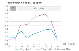
Zodiac laboratory measurement of chloramines (or combined chlorine) after adding organic matter to two pools at the same time, one treated with salt electrolysis + sand filter and the other with MagnaPool®.
