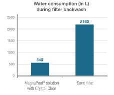
Value for a pool equipped with a 640 mm filter and a 1.0 HP (or 0.75 kW) pump.
