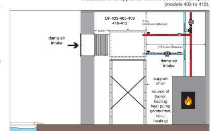
Installation of an appliance with the hot water coil option
