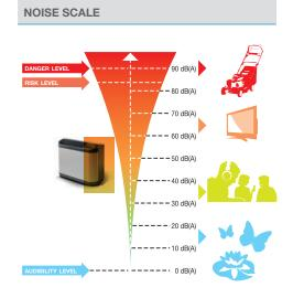
To compare the noise level of several machines, check what type of value you have, power or pressure, and if it is pressure then at what distance was it measured!
