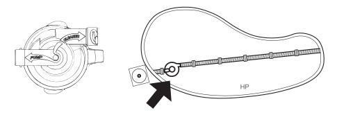
Install at the first hose connection closest to skimmer/or suction line. Ensure correct orientation using guides (Pump/Cleaner) on Leaf Catcher lid.
