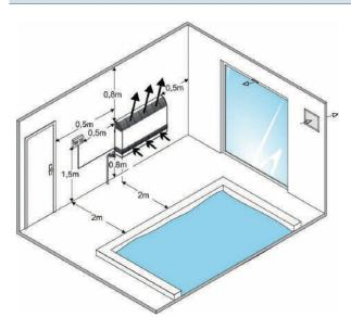
Example of an installation with a SIROCCO Free-discharge console
