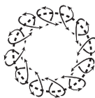
3/16" Diameter Orbit For general purpose sanding.
