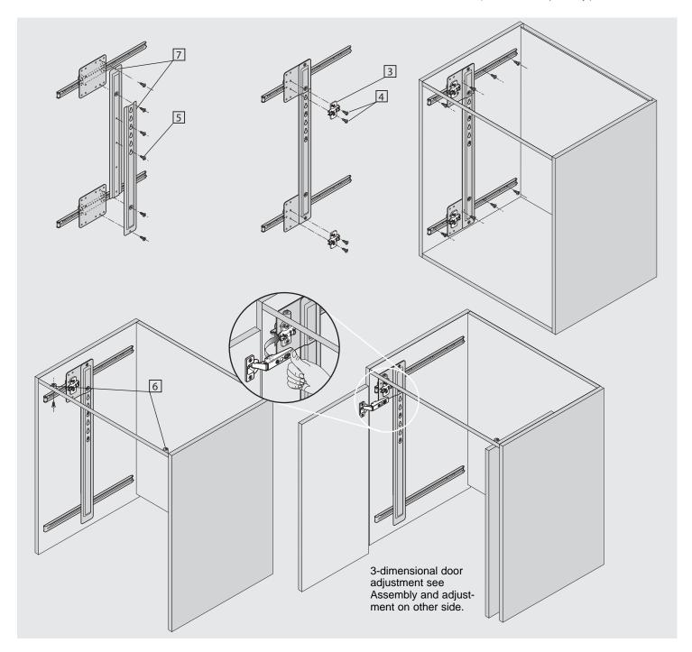
4. Attach door guides to top and bottom of cabinet with 606N or 606P screws.
