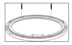
Step 6: Install the Easy Access Corner Pantry by attaching it to the inner race of the bearing with 4 ea. 1/4 - 20 X 1 flat head machine screws. Spin it and make sure it clears the inside of the cabinet and stops in the correct position
