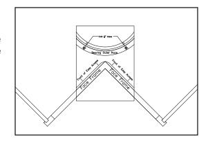
Step 2: Locate the Bearing with the bottom up, Make sure the plastic catch is engaged. Attach to the shelf with 2 - #8 x 1" Flat Head Wood Screws, through the outer race of the bearing. Make sure the screws go into the 2 holes drilled in Step 1.
