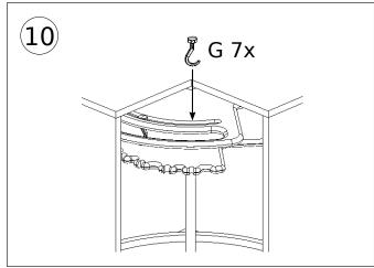
Install the (G) Hooks into the slots above,
