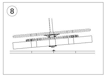
Place the pole assembly onto the bottom pin
