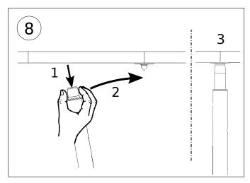
1 Pull down on the top pin, 2 locate the pole below the pin 3 Release the pin to lock into position
