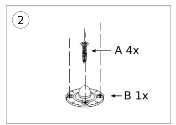
Mount the pivot bracket Top & bottom center of the cabinet
