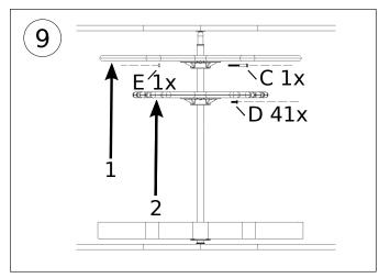
1 Raise the Top Plate assembly up, install the (E) Nut and (C) Bolt.2 Raise the Arrestor assembly up (2), install the (D) Screw and adjust height, then tighten
