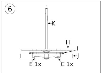
Add (J) Shelf then (C) bolt & (E) nut to secure the shelf to the (K) pole. **Tighten firmly**Slide the (I) assembly and the
