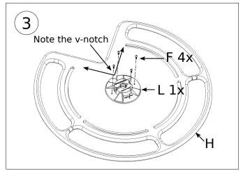
Attach the (L) pole bracket to the underside of (H) top plate. Mount bracket to the pre-drilled holes.
