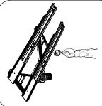
screw them in through the large access caps into tray holes (caps shown over screws holes in top half of slides (see in illustration). to slides. Then push (4) plastic screw cover the 4 holes for correct installation of tray Phillips machine screws. Illustration shows and install it to slides with four (4)  $\frac{1}{4}$  - 20 x 1" Now match a Half Moon tray over slides STEP 5
