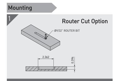
Use a  $0^{9/32''}$  router bit to cut a slot in both substrates where the Hook and Key of the Mini 60 is to be mounted. Depth needs to be 0.394'' for each.
