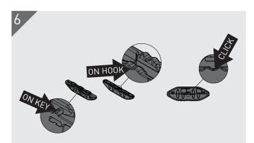
The Mini 60 features locating tabs which click into place when fully assembled. Please note this feature is not a lock, making the joint fully reversible.
