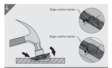
To aid in the installation of the Key and Hook, start by inserting one end in the slot when use a hammer or mallet to tap the component into place. Ensure centre lines on substrate align with centre marks on Hook and Key.
