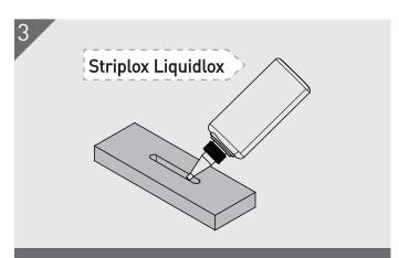
Apply Striplox Liquidlox 15 second cure adhesive to both sides of the slot in each substrate. Visit joinlox.com/ striplox or call 1800 JOINLOX to find out more about Striplox Liquidlox and Mark-Out Template.
