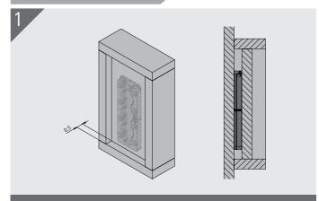
Setting back the mounting face of either the Hook (as shown) or Key by 0.5" results in a concelled joint without the need to cut rebates.
