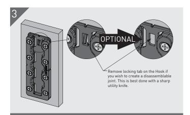
Prior to assembly, establish whether the joint is to be permanent or disassemblable.
