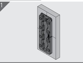
Mark center lines, vertical and horizontal, on both substrates. Flush mounting requires no additional preparation. Line the notches in each component (Hook shown here) with the center lines. Mark-Out Template can also be used.
