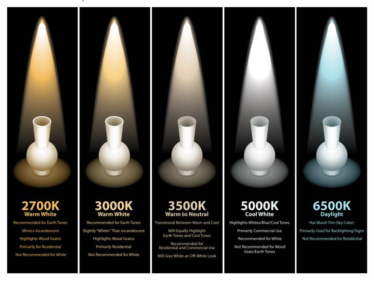
Color temperature is the rating a particular color renders on the Kelvin scale. These color temperatures alter how an object or room is perceived when illuminated and Tresco Lighting offers a wide range to choose from.
