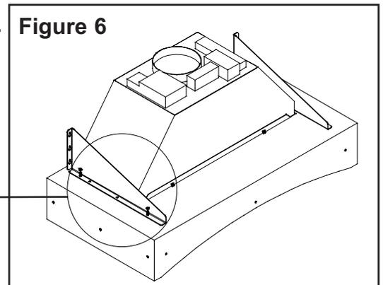
**Step 7:** Using help if necessary, lift the liner, Blower and mounting bracket assembly into position and hang on the screws extending from the mounting plate. Make sure the brackets are firmly seated into the key hole slot and then tighten all the screws (See figure 7).
