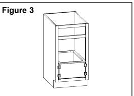
**Step 4:** Remove the Waste and Recycle unit from the cabinet and place on the cabinet door. Center on the door side to side and measure for the appropriate position vertically.
