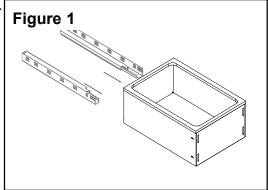
Step 2: Install 4 mounting brackets through the slots in the drawer, push them in all the way and snug the screws on the side (see Figure 2).
