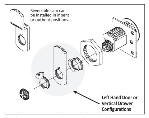
Use of cams depends on application and material thickness.
