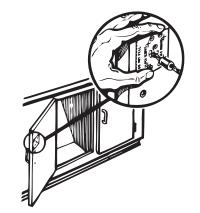
Measure door thickness, then subtract 3/16". Position drill depth gauge on bit and move it the required distance from the tip so hole drilled will be within 3/16" of cabinet door front. Drill into "7mm hole" location on guide.
