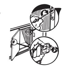
Match striking plate over 2 locations marked during step 1. Use screws and install loosely so slot adjustment can be made later. Match TOT-LOK assembly into 7mm holes (install plunger/slug if necessary), align over 4 marks (from step 2) and screw in place with four 1/2" screws. A pair of auxiliary holes are provided for variations in door panels. Assure proper position of striking plate and screw it down tight.
