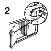
Close door firmly on foam tape. This will transfer guide to exact location on inside of door or drawer. Open door, hold guide down, and mark 4 screw locations for lock installation (4 arrows).
