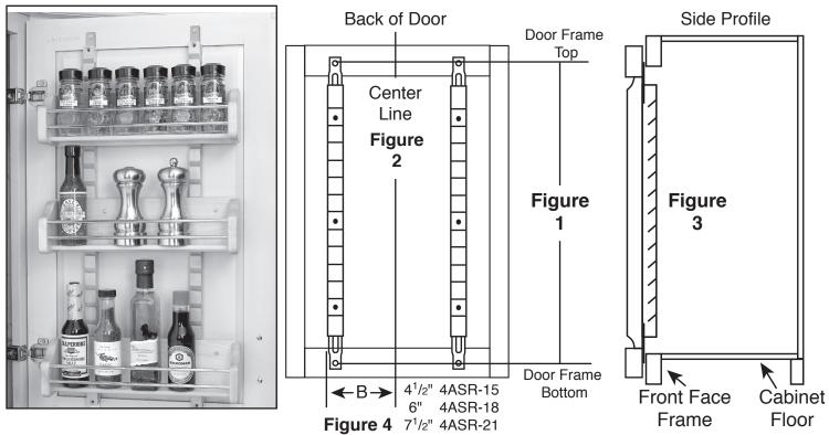
**NEW** mounting brackets adjust up to 5" so they will align in thick portion of door frame. (Standards may have to be cut to fit shorter doors.)
