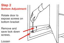
star washer screws to re-center pivot cam base (both sides). Tighten, check and repeat if necessary.
