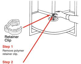
Turn adjustment wheel (located inside cut out portion of shaft) clockwise to raise shelf/door unit. One full turn raises door 1/32". After adjustment, be sure to replace retainer clip.
