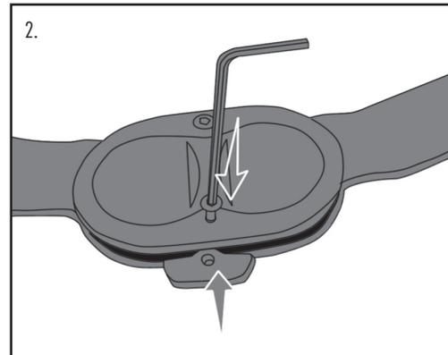
2. Choose the stop with the desired degrees of extension and install it on the extension stop side of the hinge. Be careful not to overtighten the screw and strip the hole.
