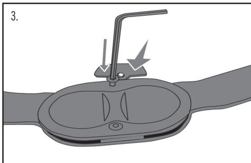
3. Choose the stop with the desired degrees of flexion and install it on the flexion stop side of the hinge. Be careful not to overtighten the screw and strip the hole.
