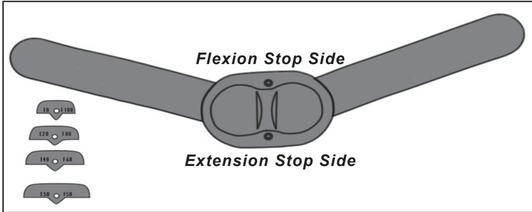
Extension stops are available in 10 degree increments from 0 to 50 degrees.
