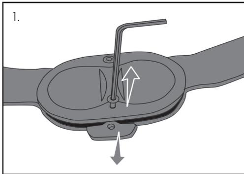
1. Use the included hex wrench to remove the existing hinge stops by removing the screws on both the extension stop side and flexion stop side of the hinge cover.
