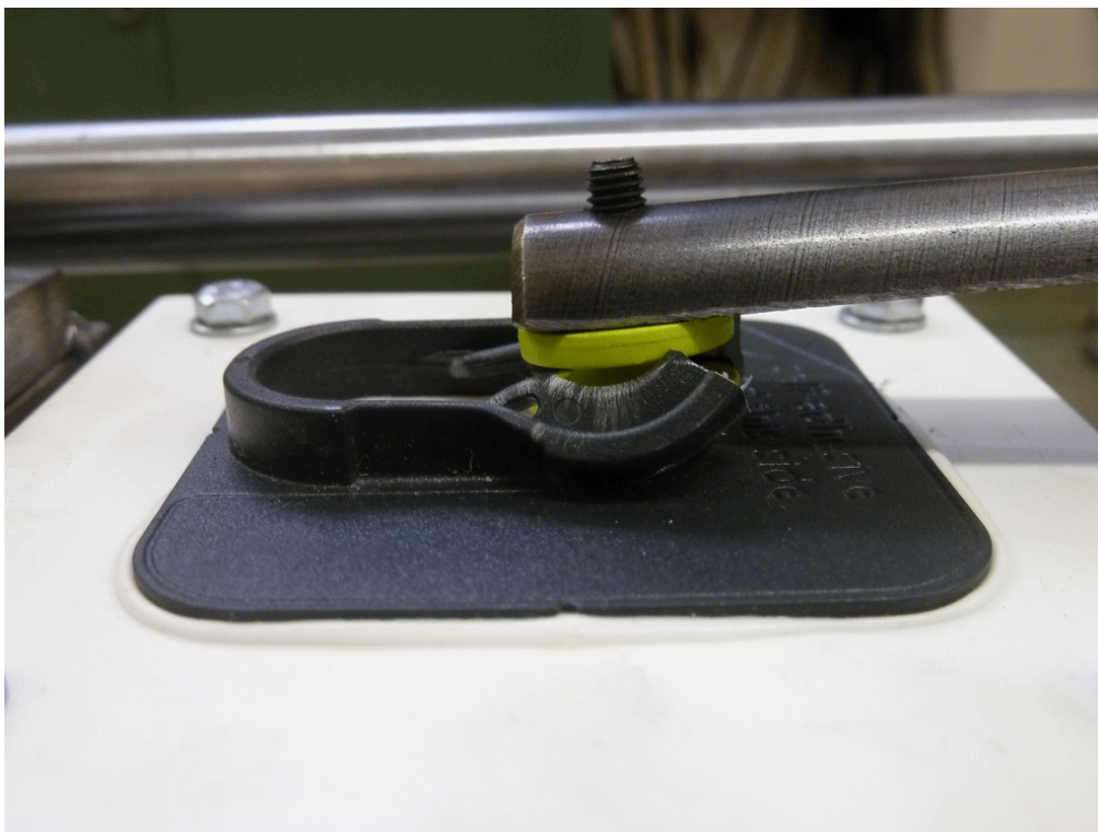
Photograph 2 A view showing vertical (shear) failure mode. The mount material surrounding the button distorted and the button pulled from mount.
