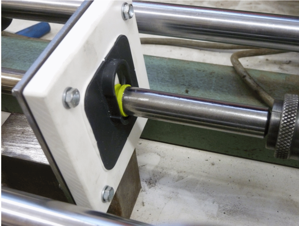
Photograph 3 A view showing the test set up for surface mounted 85 degrees from vertical (tension) test.
