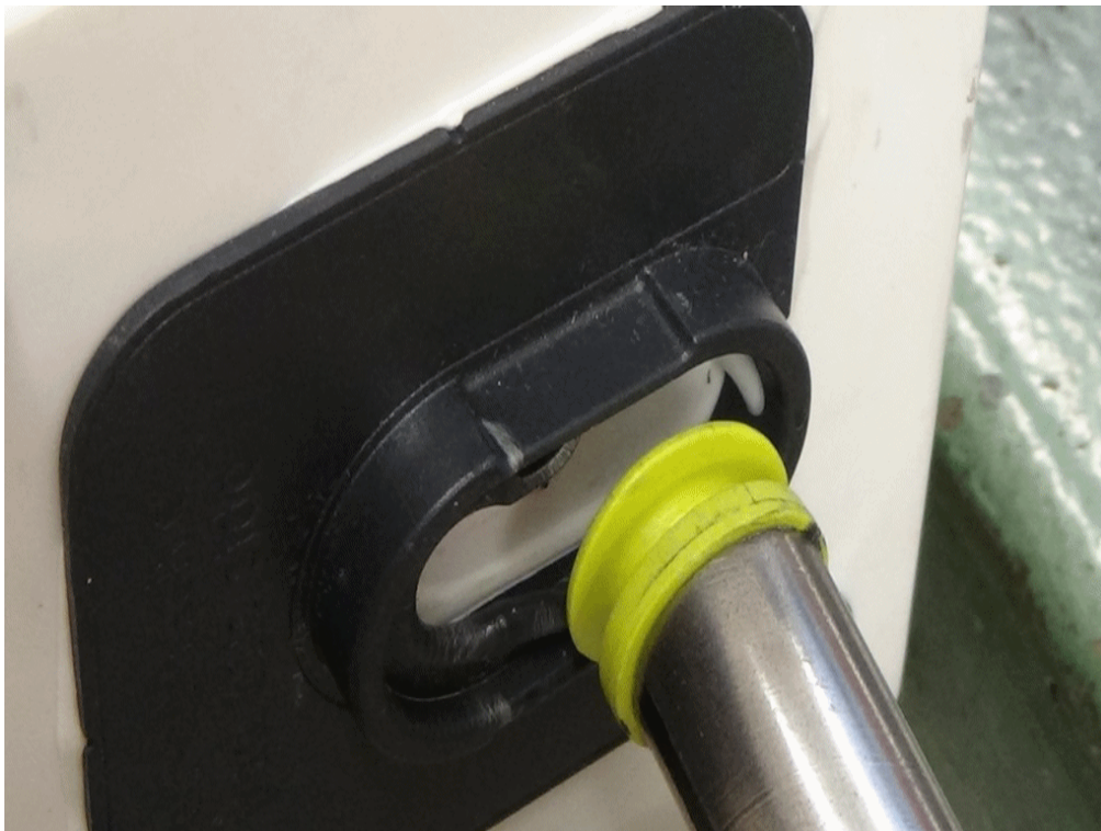
Photograph 4 A view showing the 85 degrees from vertical test failure mode. The mount material surrounding and the button distorted, allowing the button to be pulled from the mount.
