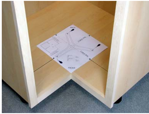
2. Put in the drilling template
