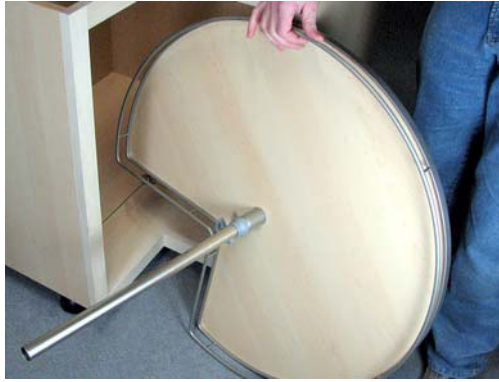
2. Put the bottom shelf on the axle
