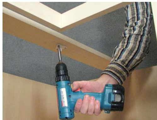
2. Screw the upper bearing
