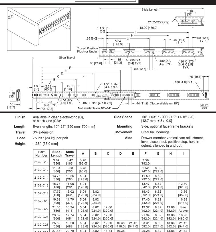
Load rating based on an 18" slide in a 16" wide drawer cycled 50,000 times.
