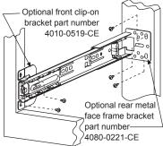
4180-0321-XE. Each kit contains: 2 front brackets 2 rear brackets, and installation instructions. Order 1 kit per pair of slides.
