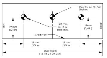
STEP 2: USE #8-32 x 1inch SCREWS TO ASSEMBLE
