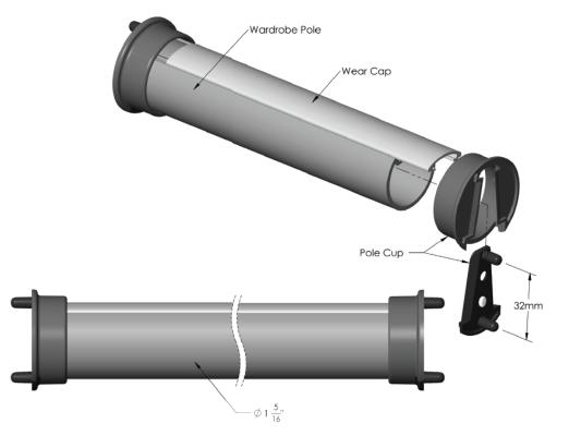
\*Note: For cutting, pole should be oriented with the wear cap facing down:
